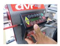
Re fix New Control Panel and switch on power and test New Control Board.
