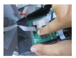
Plug in Motor Controller Cable to New Interface Panel. Make sure it is firmly pushed home in socket.
