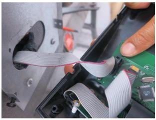
Disconnect the Motor Controller Cable
