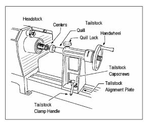
The Nova 3000 lathe incorporates a unique adjustable tailstock to ensure the utmost in turning accuracy.
