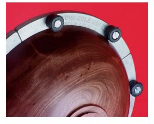
The Cole Jaws (both Std and Mini sizes) are some of the most popular of the Chuck accessory jaw sets in the Nova Range. They are a fast, easy way to re-chuck bowls.
