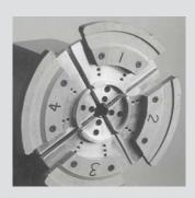
Jaw segments can be made from Medium Density Fibreboard (MDF)
