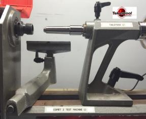
Tighten the bolts inside the headstock on each side then remove the Acruline gauge by Un-locking the Tailstock from the bed and then using a Knock-out bar, tap the acruline gauge out of the Headstock spindle, then do the same with the Tailstock. The spindle of headstock and Quill of the tailstock should now be on the same centreline.
