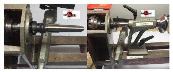
Clean out the Morse tapers in both the Headstock and Tailstock spindles. Fit the 2MTNA acruline gauge into the headstock spindle and tap with a soft-faced mallet or a piece of wood to "drive it home". Bring the tailstock up to the Acruline gauge and fit it into the Tailstock spindle by driving the tailstock into the taper. Lock the tailstock to the bed.
