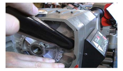
4. Try sucking the dust through the vent at the front of the Headstock under the spindle. Again position the nozzle at different angles to suck as much dust through as possible.
