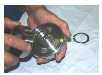
Place scroll ring in chuck and move it counter-clockwise till it has engaged. Make sure the jaws have not moved and still have a square form in the centre.
