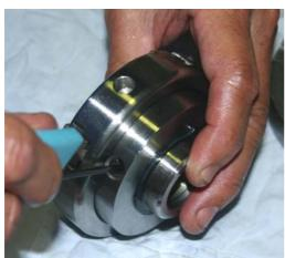
Using circlip pliers to insert the circlip back into the groove above the scroll ring.
