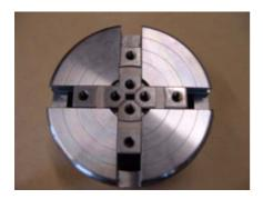
Push all jaw slides to meet in center forming a square. Make sure the No. 1 Jawslide is in the slideway with the dimple (a small half moon shape on the inner diameter of the slideway)
