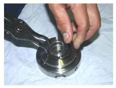
Do not worry if there is no grub screw in the chuck. It is not used in all chucks. Extra grub screws are supplied in the packing if it is needed at a later stage
