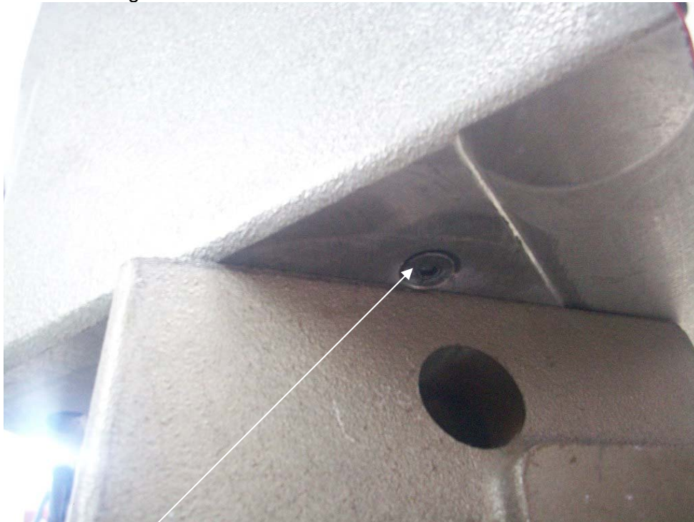
Screw exposed by swivelling head stock around
