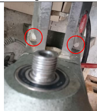
Figure 3: Bolts connecting the bed to stand
