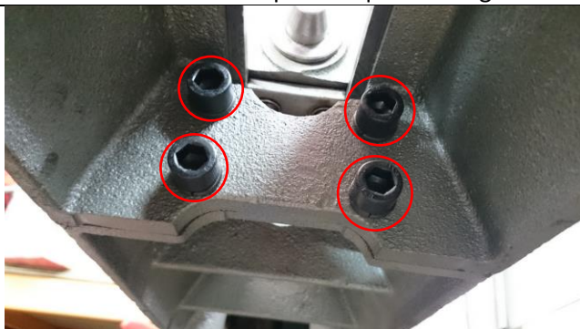
Figure 2: Bolts connecting the beds
