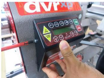
Re fix New Control Panel and switch on power and test New Control Board.
