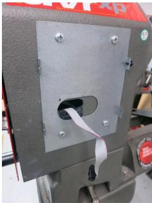
Control Board (Interface Panel) disconnected from Motor Controller Cable
