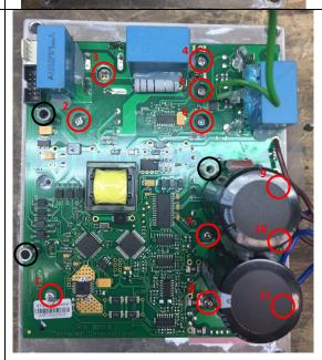
**6.** Remove the control board.
