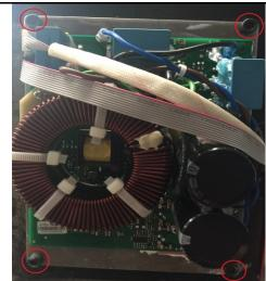
**4.** Remove the coil from the control board.
