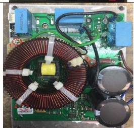
Remove the three coil support posts by hand (circled in black).
