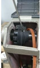
You should be able to slide the pulley along the spindle shaft with your hands.
