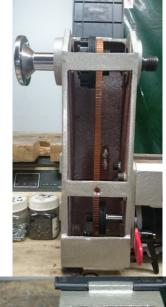
Carefully remove the belt from the pulleys so the position will not change and return the grub screw back to secure.
