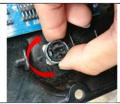
**5.** Replace the switch with a new one. The assembling procedure is the exact opposite of disassembly.
