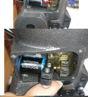
**5.** Remove the gear and the insert block (the black block).
