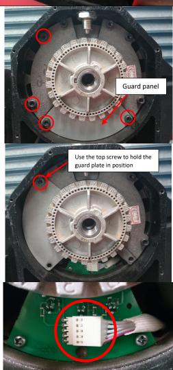
4. After checking every cable connection, assemble everything back together lightly and retry the lathe.
