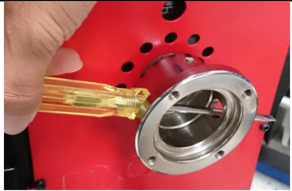
Figure 3: Screwdriver in handwheel to lock in place
