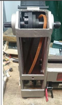
Remove the grub screw which is holding the spindle pulley in place.
