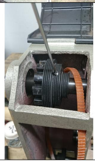
Put the belt back onto the desired position.
