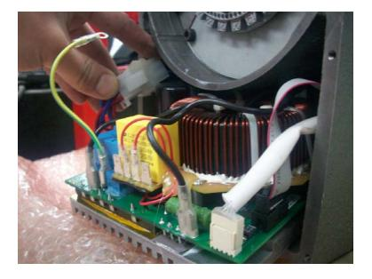
Feed the control board <sup>3</sup>/<sub>4</sub> of the way in and plug the 6 pin stator wiring plug into the corresponding plug on the control board. Attach the sensor cable and the ribbon cable into their corresponding sockets on the control board.
