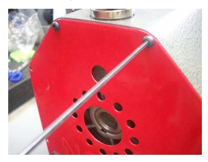
9. Position the control board panel on its bracket and fasten the 4 screws on the sides.
