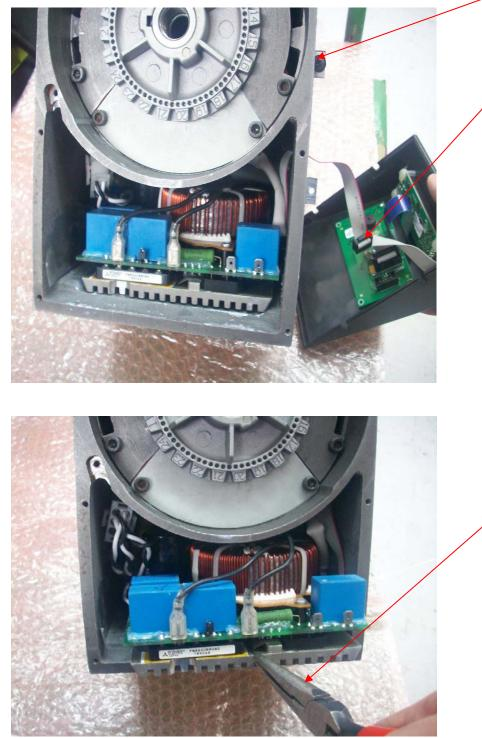
Unfasten these a few turns to release the control cover. The ribbon will be connected and will have a blob of glue bonding the plug and receptacle together. The glue can be pulled off and the ribbon plug removed. Feed the ribbon plug back through the hole on the side avoiding any scraping on the ribbon.
