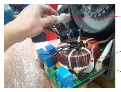
Disconnect the 6 pin white plugs thus separating the stator wiring from the control board.
