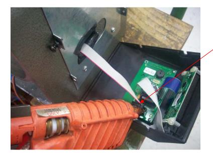
Glue the sides of the socket for the ribbon cable and then
