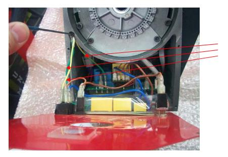
The three earth wires must be connected together and be fastened into the inside of the headstock casting.
