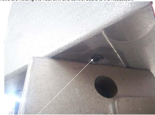
Screw exposed by swivelling head stock around
