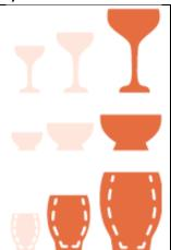
Designed for expanded dovetail, reverse dovetail and for gripping footed bowls, this is one of our most popular jaws mount 12-14" bowls. It can also mount false wooden jaws, so customised jaws can be made for special purposes.
