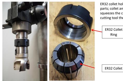
ER32 collet hold the cutting tool by using 2 main parts; collet and collet ring. The collet ring squeezes the collet ring which then squeezes the cutting tool therefore holding the tool in place.
