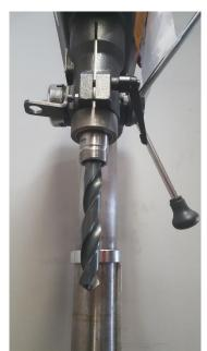
1inch brill bit with MT3 mounted directly into the spindle
