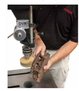
A user-friendly LCD screen allows the user to access a picture menu, a feature generally found only on CNC machines. The user can select the drill bit they want from the menu, then select the size and the material they are drilling into, and the computer will select the correct speed.
