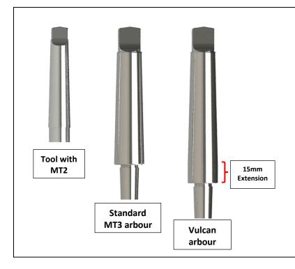
Image on the side compares the drill chuck arbour for the Vulcan against the standard MT3 arbour and MT2.
