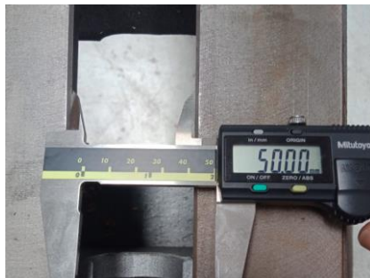
Minimum space between lathe bed rails 1 (Left) and max width of alignment plate (right)
