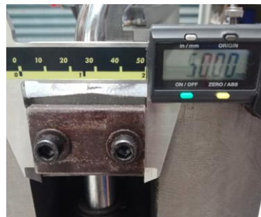
Minimum space between lathe bed rails 1 (Left) and max width of alignment plate (right)
