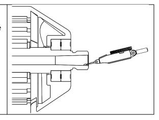
A 150mm faceplate (FP150L) is used as the NOVA standard to test if the runout is caused by the spindle thread or the tool which is attached. Before testing, make sure to correctly screw on the face plate:
