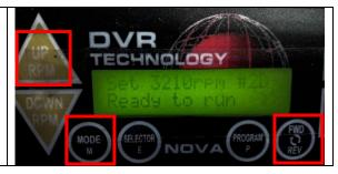
4 Using the **<UP RPM>** and **<DOWN RPM>** buttons, enter the password "**3210**".
