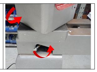
3 Unbolt each heat sink screws exposed underneath the headstock when rotated.
