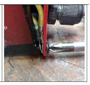
11 Attach the HMI ribbon to the new HMI panel and attach it to the headstock before screwing it on.
