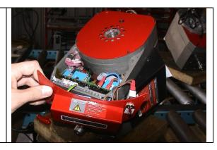
5 Carefully use your long nose pliers to begin to remove the control board by pulling on the heat sink. Be careful not to touch the control board with your pliers.
