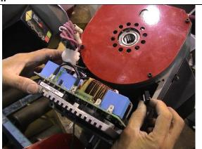
9 Replace the four Allen screws underneath the headstock to secure the control board in place.
