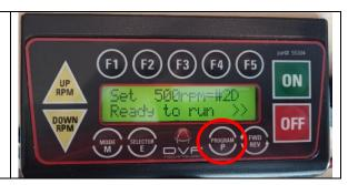
2A Press the **<Selector E>** key to cycle through the vibration sensor settings.
