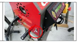
3B Power the lathe on again for 30 seconds before turning it off again to complete the factory reset.
