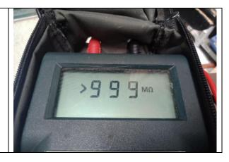
Repeat this step for all 6 motor-side pins. Take note if any windings have a low insulation resistance.
