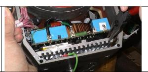
4 Disconnect the motor cable by pinching the buckle and separating the connectors.
