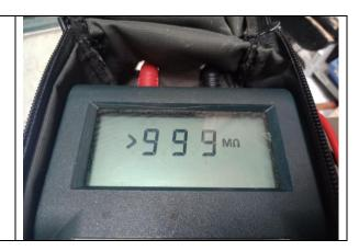
If you have a multimeter, you can also check if the AC terminals have shorted internally by setting the multimeter to resistance mode, and touching the two probes to the two AC power terminals.
