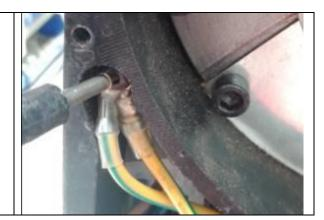
Touch the other probe onto one of the 6 pins on the motor side of the cable.
