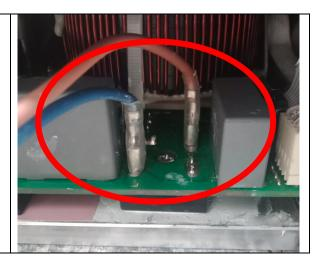
Check that the green & yellow earthing cable is secured to the headstock
