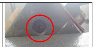
4 Unscrew the 8 screws holding the headstock cover plate on to expose the main control board.
