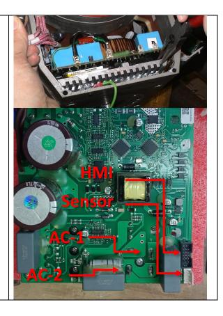
Unplug the 6-pin motor cable by unbuckling the belt and separating the connectors.
