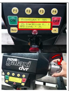
7 Press the **<OFF>** button and then turn the lathe off to clear interim settings.
