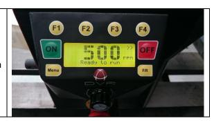
2 Press the **<Menu>** button and rotate the speed dial until "Service" is selected.
