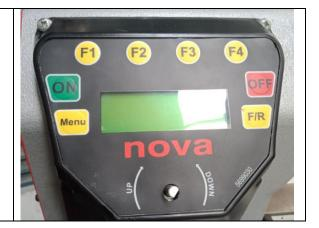
5 Replace the speed knob back onto the HMI and secure it with the grub screw.
