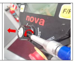
3 Using your flat head screw driver or a scraping tool, peel the keypad membrane off from the HMI panel.
