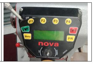
4 Peel the film off the back of the new keypad and carefully apply the membrane onto the HMI panel surface.
