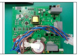
8 Attach the 6-pin stator cable, sensor cable, HMI control ribbon, and AC power leads to your new MCB as you are inserting the board into the headstock.
