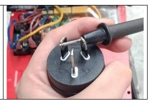
12 Unplug the two AC power leads from the main control board.
