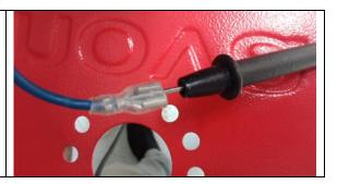
13 Replace the power leads onto their spade terminals (in any polarity) and screw the cover panel back onto the headstock.
