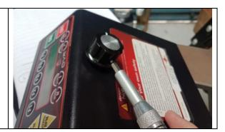
With some pliers undo the nut holding the old rotary encoder to the HMI panel. Remove the washers too.
