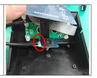
8 Screw the nut and washers back to the rotary encoder on the other side of the HMI panel to secure the encoder in place.
