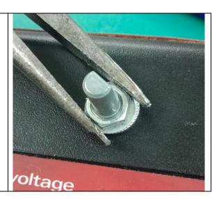
6 Remove the screws holding the HMI circuit board in place.
