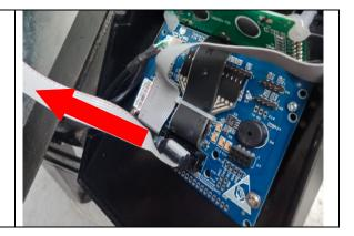
4 Using a small flat head screw driver, loosen the small grub screw inside the speed knob and slide it off the encoder shaft.
