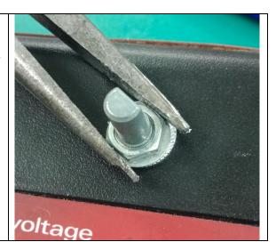
9 Fasten the four screws to secure the HMI circuit board back to the panel
