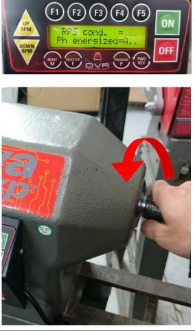
6 Press the **<OFF>** button and then turn the lathe off to clear interim settings.
