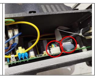
4 Cut the cable tie which ties the main power cable and sensor cable from the motor to the main board.
