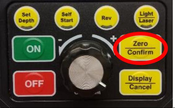
A close-up photograph of the control panel for a NOVA Viking depth sensor. The panel is black with several buttons: 'Set Depth', 'Self Start', 'Rev', 'Light Laser', 'ON', 'OFF', 'Zero/Confirm', and 'Display/Cancel'. The 'Zero/Confirm' button is circled in red. |
