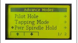
Press the **<ON>** button to activate the spindle hold function. The screen will display a countdown for approximately 30 seconds and the motor power.
