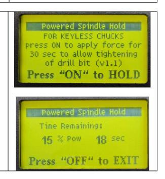
3 After the countdown has reached 0, the HMI will reset back into the main idle screen.
