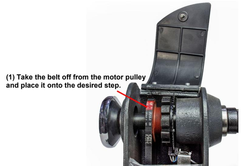
1. Place the belt onto the desired spindle pulley once the belt is removed from the motor pulley.
