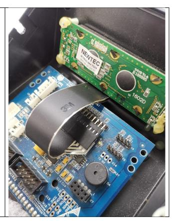
Plug all the remaining wires back into the circuit board.
