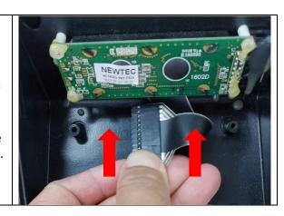
6 Insert the new keypad by twisting the connector in the same way.
