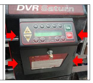
3 Unplug the external stop and the 10 pin ribbon cable from the headstock.
