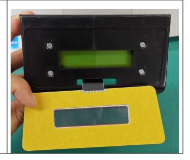
7 Place the circuit board back into the panel. Make sure the keypad cable is between the screen and the blue board (as shown)
