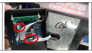
4 Undo the 4 screws and remove the circuit board.
