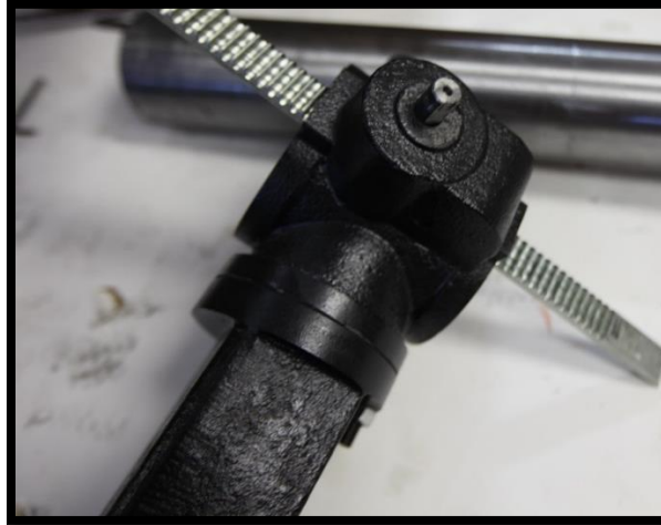
Figure 3 - Mounting the table bracket and rack 1/2
