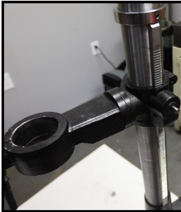
Figure 4 - Mounting the table bracket and rack 2/2
