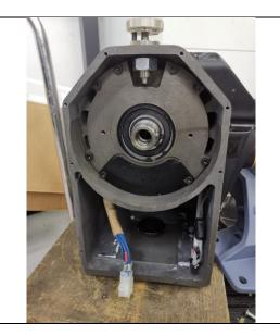
2 Locate the large 6 pin motor connector on the motor side.
