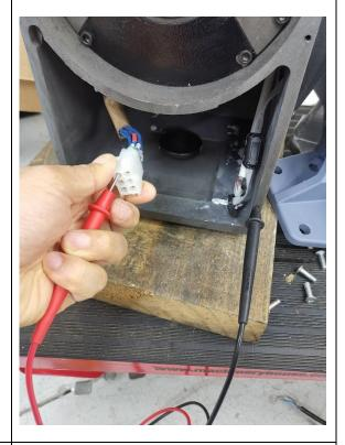
Set the multimeter on continuity mode or resistance mode and check if any of the 3 phases is shorting to the main casting. Repeat for all 3 phases.
