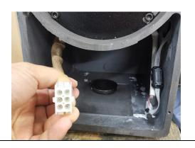
3 The motor winding has **3 pairs** of phases.
