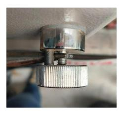
3 Unwind the knurled cap of the spindle lock by rotating it counter clockwise
