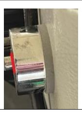
5 Screw the knurled knob to the marked line and test if this is able to lock in the correct position
