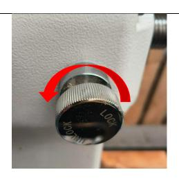
4 Using a marker, mark the position of the locking pin when the spindle is locked.
